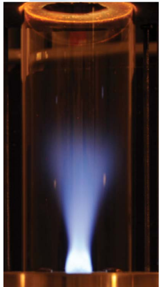
Figure 1: Visible Light Image of Lean Direct Injected Hydrogen/Natural Gas Flame
