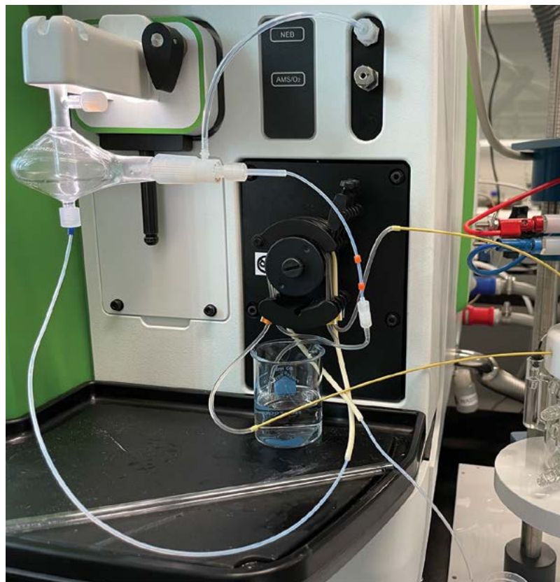
Setup for In-Situ Monitoring of Catalyst Dissolution with ICP-MS Elemental Analysis
